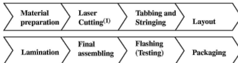
(1) Laser cutting is only necessary for smaller-sized modules.
